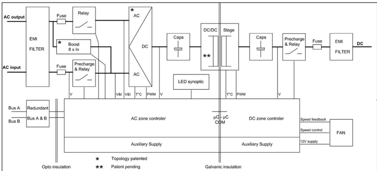
ECI technology has AC to DC, DC to AC, and DC to DC converters to provide constant and disturbance-free output power regardless of the input source.
