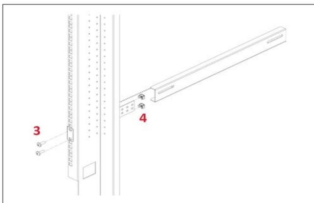
Assemble the sliders and adjust the length to suit the mounting depth.
