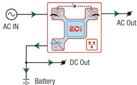
The total output power of a module can be shared between the AC load, DC load and charging power based upon the requirement.
