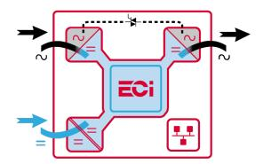
The ECI technology **eliminates all single points of failure** with full scalability; up to 32 modules in parallel and high efficiency of above **93.5% in DC/AC conversion**, hence reducing operating costs. We can build the systems up to **2.7 MVA.**
